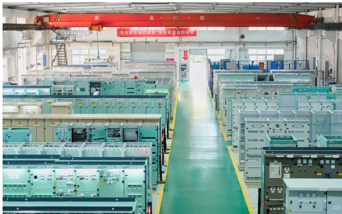
LV Switchboard Workshop
